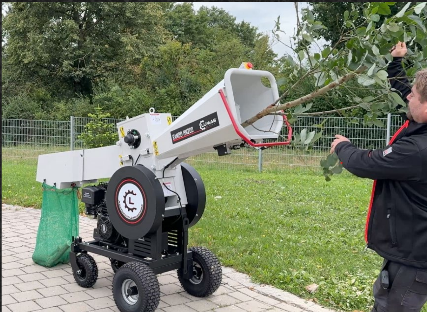
Chassis with parking brake and drawbar.
